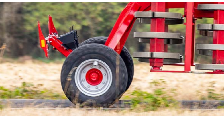
Transport chassis Safe road transport, optional brake system
