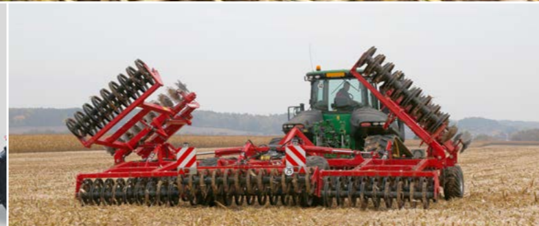
Transport chassis Safe road transport, optional brake system
