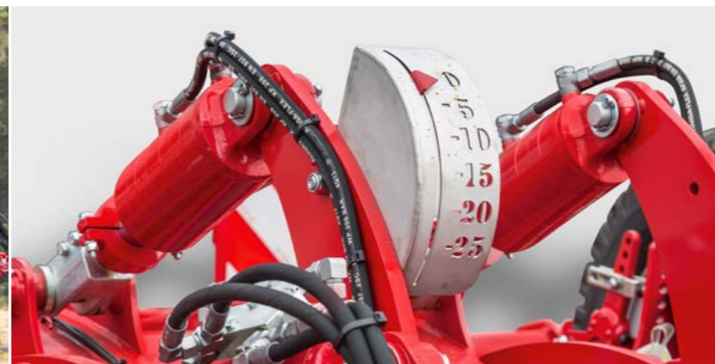
Optional For Joker 5/6/8 RT hydraulic working depth adjustment
