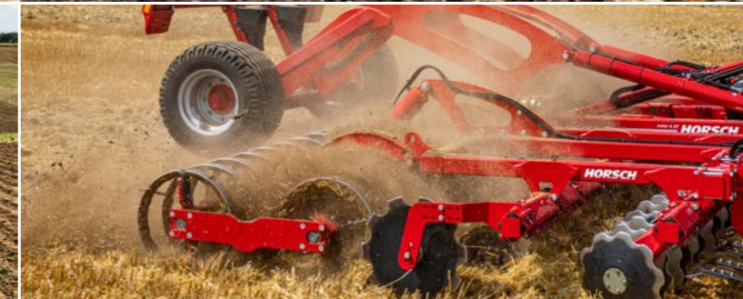
Effective packing system ensures intensive crumbling and consolidation.
