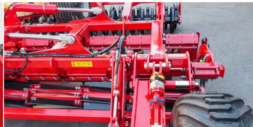
Working depth adjustment with clips (standard)
