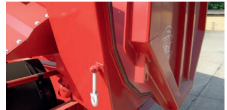
The sealed tailgate makes for safe hauls of wet material.
