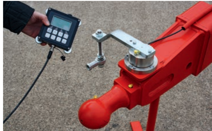
The electronic forced steering system allows operators to select one of many programs that control the trailer's response to their steering.
