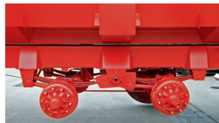
Running gear comprising 24 t – 32 t parabolic springs with axial arms and axles spaced at 1.36 m or 1.55 m.
