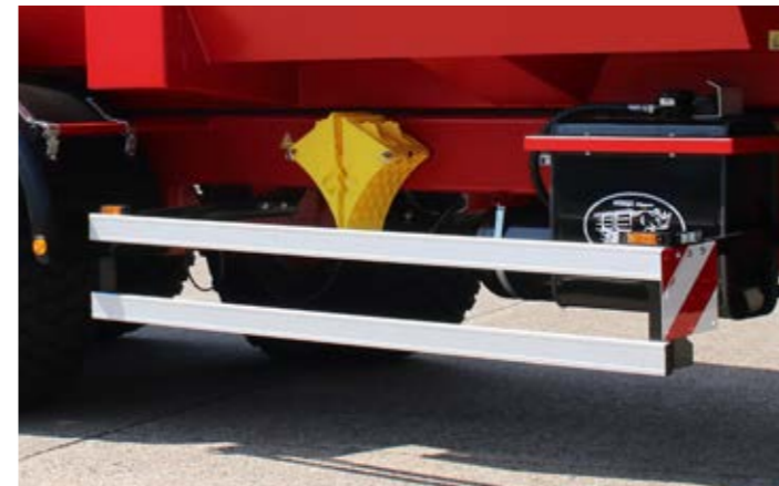
The optional side guard improves road safety and is a statutory requirement in many countries.
