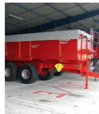
The roll-over sheet is attached to the body itself. Silage sides are no problem.
