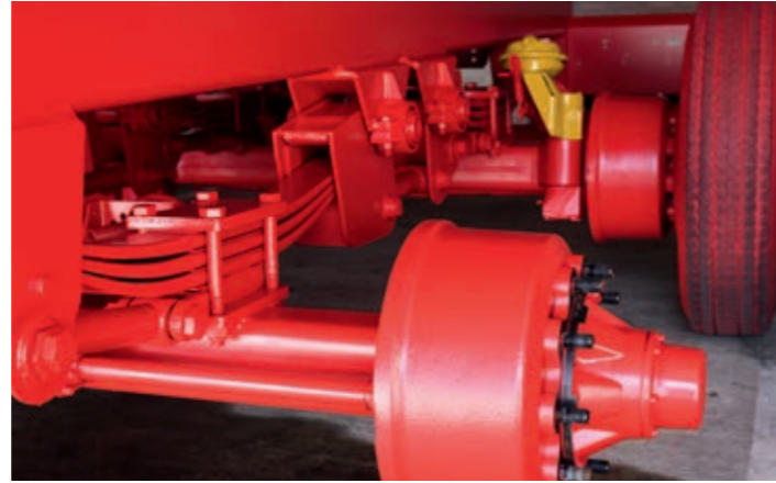
Krampe modified the brake cylinder of the ADR steering axle which leads to superior ground clearance and protection to the diaphragm cylinders.
