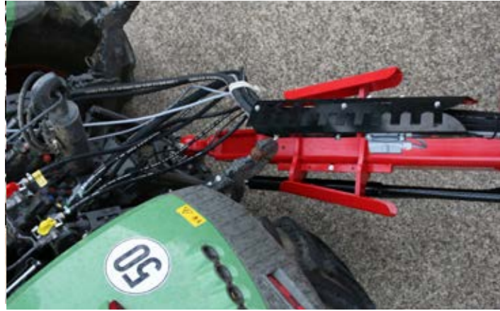
The extremely slim drawbar assembly makes for very tight turns. Forced steering ensures your trailer tracks perfectly behind the tractor – when travelling at speed, in boggy terrain and during reversing.
