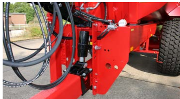
On demand, the vehicles can be equipped with a hydraulically height-adjustable drawbar.
