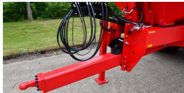
The ZV 22 drawbar with two in-line rubber blocks offers a tongue load of up to 4 tonnes.
