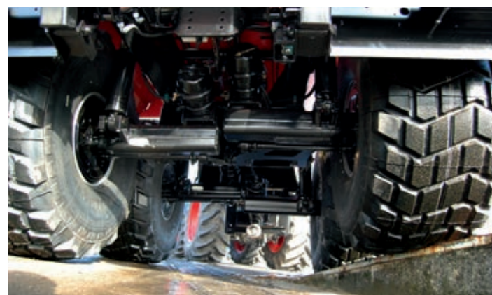
Just another typical Krampe innovation – axles with true independent wheel suspension and connectable suspension via nitrogen dampers.
