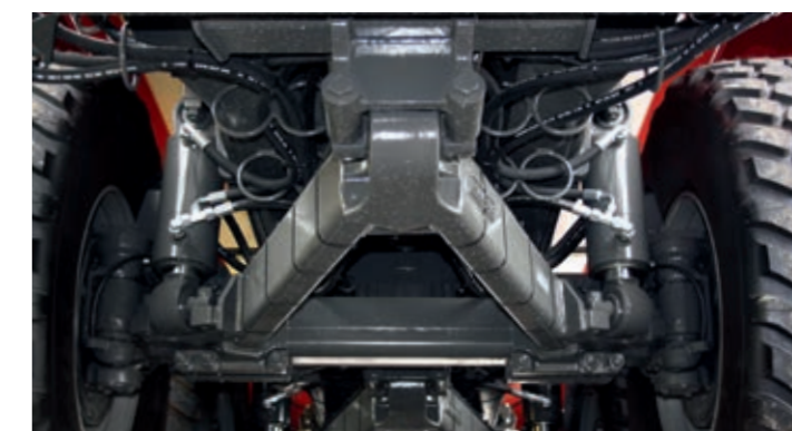
Option: The advanced Tridec running gear results in light pulling and great adaptation to difficult terrain. Measuring only 2.55 m in overall width, it still features forced steering and 600 tyres.
