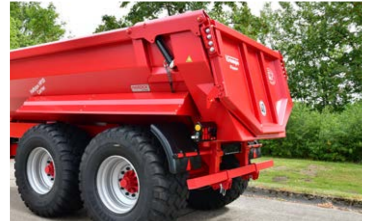
Option: The underide guard swings up to give optimum ground clearance in difficult terrain.
