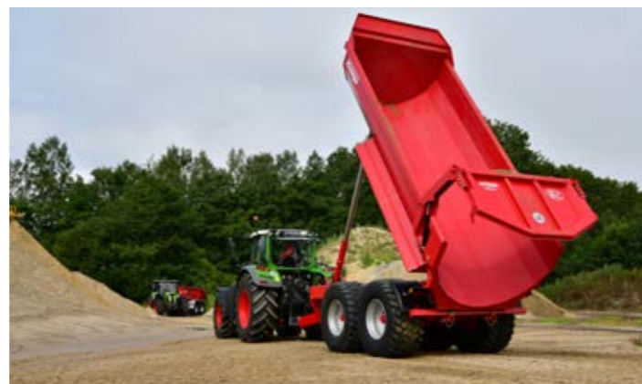
Naturally, the tailgate also opens clear if necessary.
