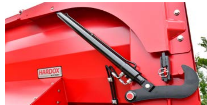
Better seal of the tailgate trough locking hooks and a lock-pressure valve.
