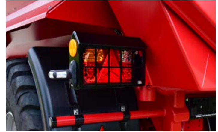
Pointed roof covering prevents dirt from collecting on the rear lights. Grids give protection and flexible position lamps provide added safety.
