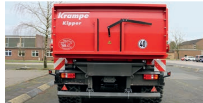
The tailgate on our SK models can be equipped with an optional outlet slide for controlled and consistent unloading.
