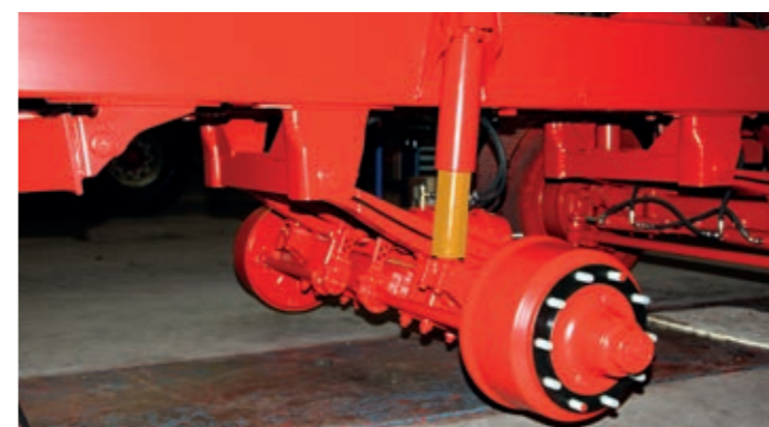
Few manufacturers have the experience we have in building hydraulic running gears. The standard guard tubes protect the chrome-plated piston rods from damage from stones.
