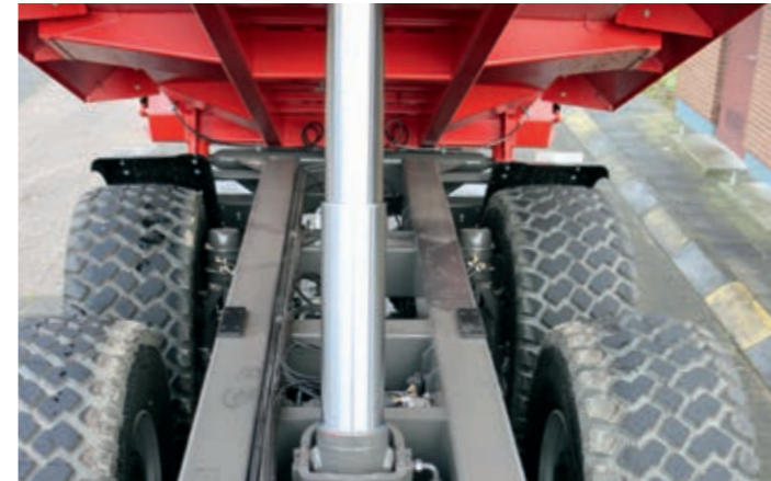
The telescoping ram features a gimbal ring and a tap. Cross braces and oversized traverses bring the necessary rigidity to the structure.
