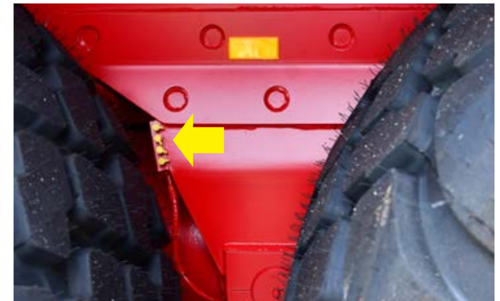
Machines with walking beam running gear or independent hydraulic wheel suspension have a lubrication bank that attends to all greasing points, especially those in awkward positions.
