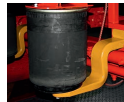
Massive pneumatic bellows mounted on cranked holders bring exceptionally quiet running to our heavy-duty Tridem tippers. Bleeding takes place automatically during tipping.
