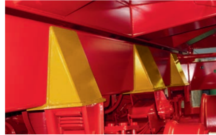
The leaf springs are generously spaced to enhance machine stability on the rough, an asset not only in rough terrain but also if the machine's centre of gravity is high.
