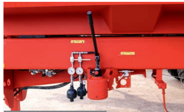
Manual pump for forced steering You can apply pressure to the forced steering with the hand pump. A manometer enables monitoring the pressure.
