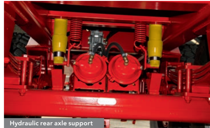
Hydraulic rear axle support The hydraulic rear axle support system comprises two rams that extend towards the rear axle during the tipping process, thereby eliminating any negative tongue load on the tractor's rear axle and thus any risk of the tractor end rearing up.
