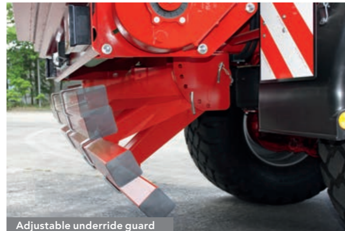
Adjustable underride guard The adjustable underride guard offers a flexible ground clearance that is adjusted without tools.
