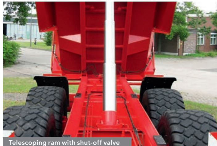
Telescoping ram with shut-off valve The telescoping rams feature gimbals rings and taps. Cross beams and traverses add rigidity to the structure.
