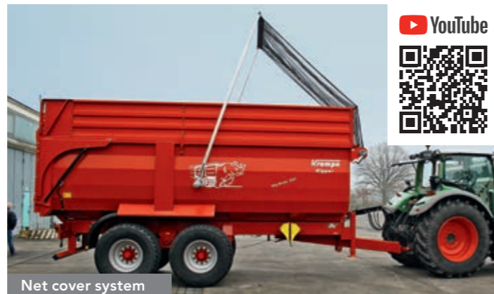
VBK covers The lateral foldable system offers a quick cargo covering.
