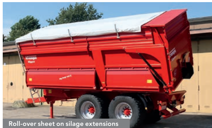
Roll-up cover Roll-up covers have always performed well on short bodies.
