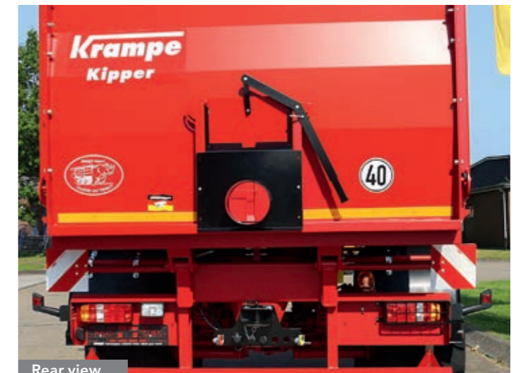
Rear view The trailer's rear featuring an automatic hitch, air and oil connectors, rear light guards and position lights.
