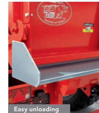
Easy unloading The chute plate is a big help when dumping potatoes into the hopper.
