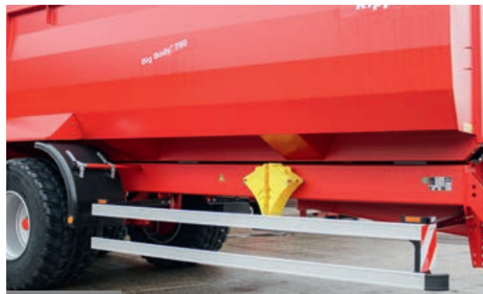
Side guard The side guard increases road safety and is a statutory requirement in many countries.
