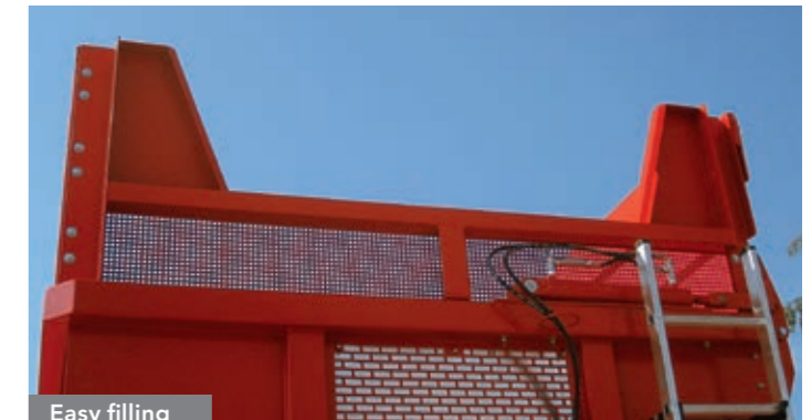
Easy filling The top of the headboard is V-shaped, offering easier filling when the trailer is following behind the forager.
