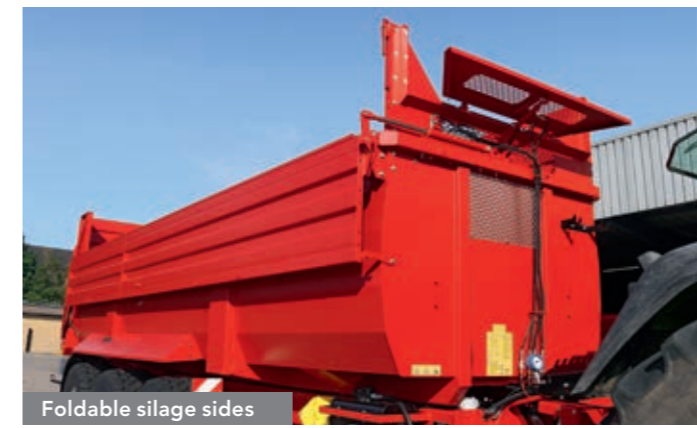
Alternative silage sides The silage extensions are available as aluminium profile with a height of 40 cm or as steel profiles with a height of 60 or 80 cm.
