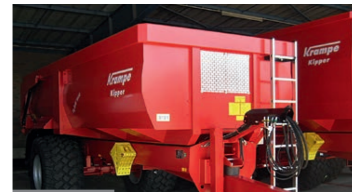
High top frame A 200 mm top frame increases capacity without fitting extensions.
