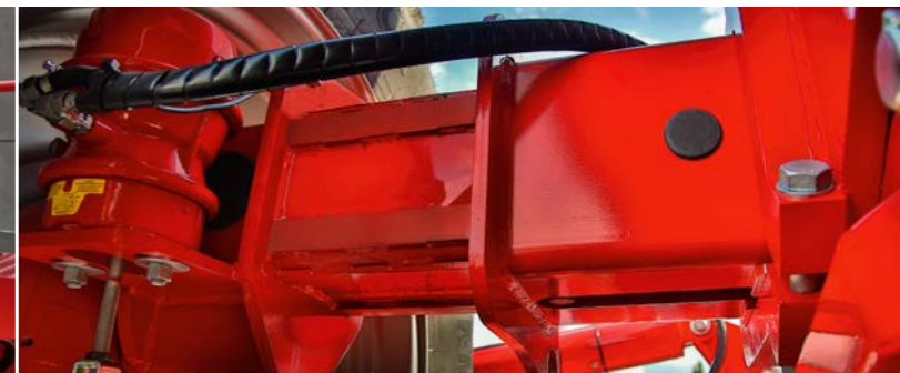
Standard telescopic axle Compact transport width; reduction of the track pressure behind the tractor track
