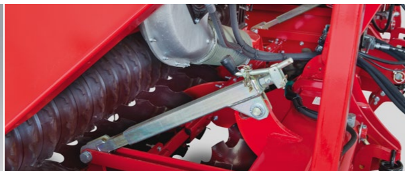
Depth adjustment DiscSystem via two adjusters. Optional: can be made while driving via two hydraulic cylinders.
