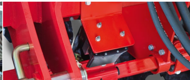
Radar sensor for an exact recording of the speed and to control the seed quantity
