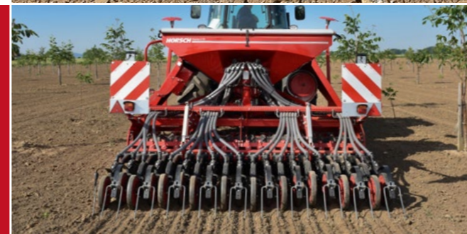
Seed hopper with a capacity of 1 500 litres
