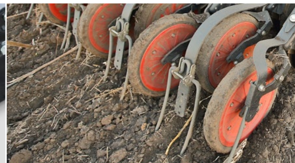
DoubleDisc coulters Straight discs with inner maintenance-free bearings
