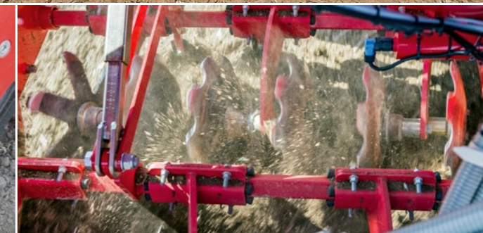
DiscSystem for intensive cultivation. Resistant even to high amounts of organic material.
