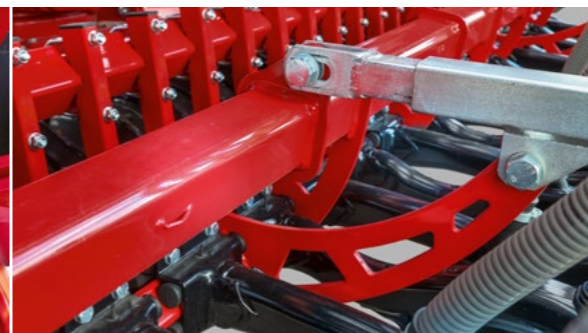
Stepless coulters pressure adjustment Manual adjustment increases the pre-load of the rubber elements
