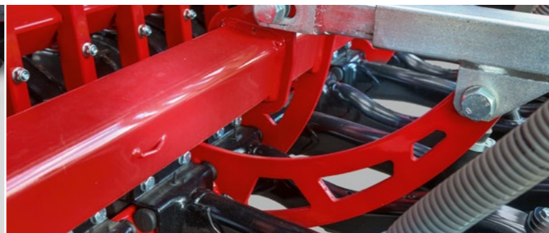
Continuous coulter pressure adjustment Manual adjustment increases the pre-stressing of the rubber elements
