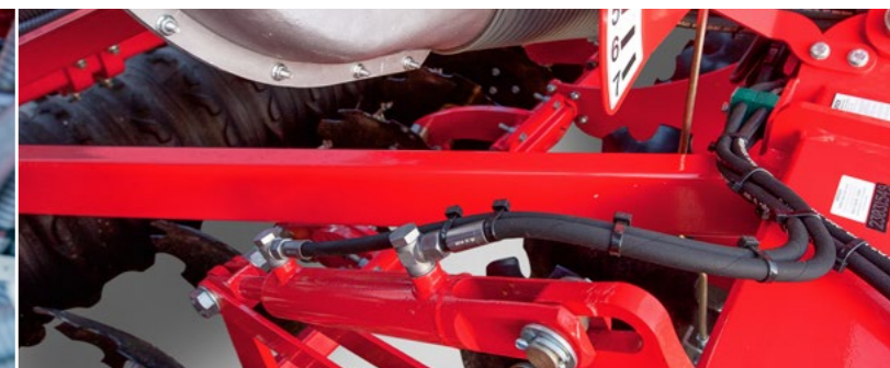
Hydraulic depth adjustment DiscSystem (optional)
