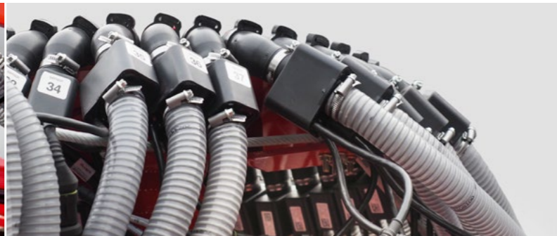
Blockage monitoring sensors for seed and fertiliser
