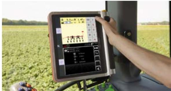
With e-drive II each sowing unit is driven individually via an electric motor. All the data is entered and read by an ISOBUS conform terminal like IsoMatch Tellus. The sowing distances are infinitely adjustable on the move. All the sowing units can be switched off individually. This solution saves seeds and money!
