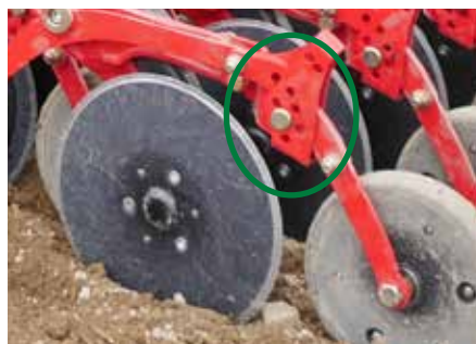
Flexible press wheel setting
