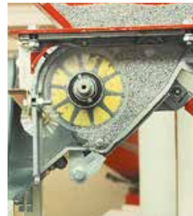
Setting for fine seeds, with rotary brush
