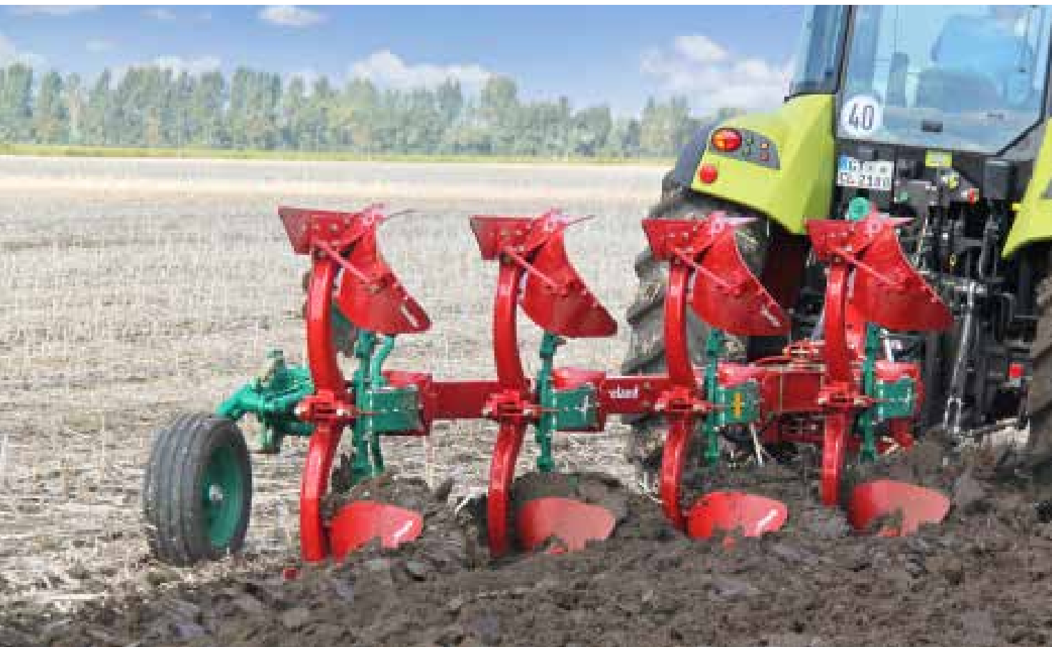
Kverneland 150 S with Auto-reset (s= spring)
