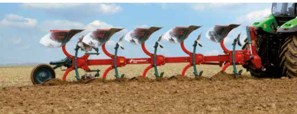
Kverneland 150 B with shear bolt protection (B=bolt)
