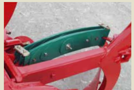
Double spring package - with 14 leaves (1400 kp)
