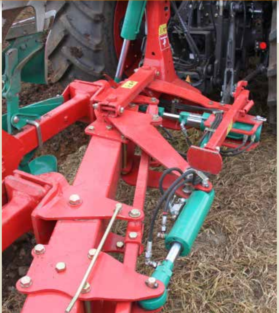
Parallel linkage with memory cylinder and hydraulic front furrow adjustment
