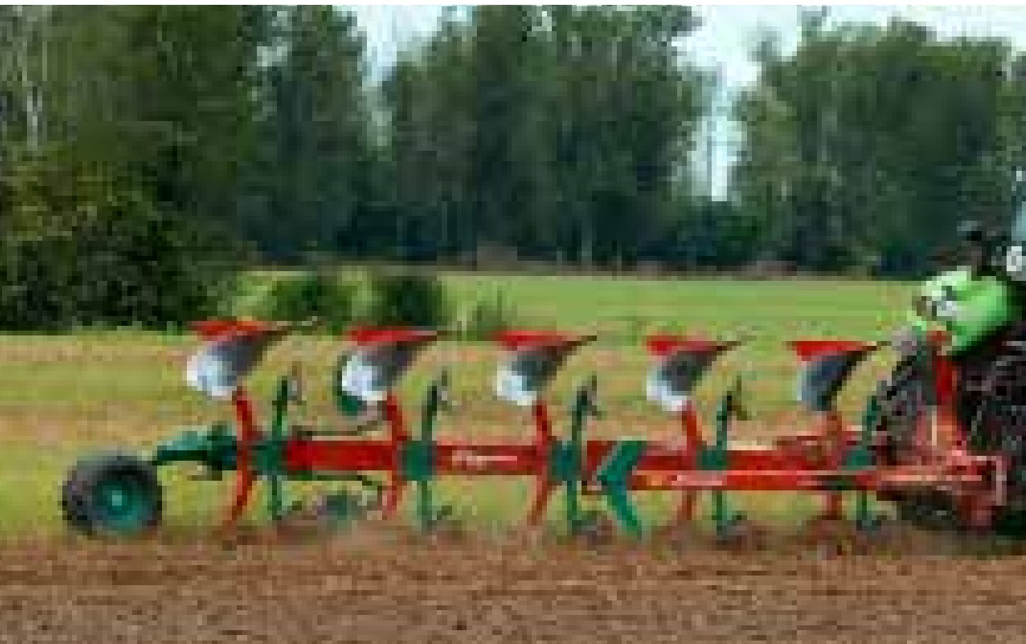
Kverneland LB 100 with spring loaded packer
