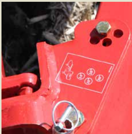
Manual working width adjustment (Kverneland 150 B/S)
