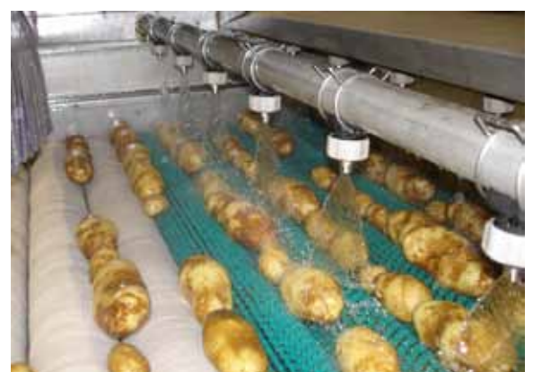
Potatoes going through a Wyma Flat Bed Modular System with spray bars
