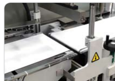
Sealing heading designed to avoid dirt accumulation
