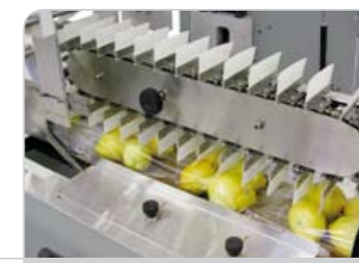
Overhead conveyor for controlling groups of products
