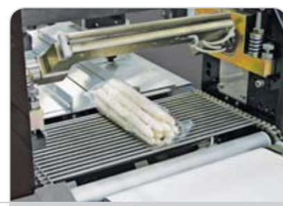
Motorized carrier through the sealing jaws
