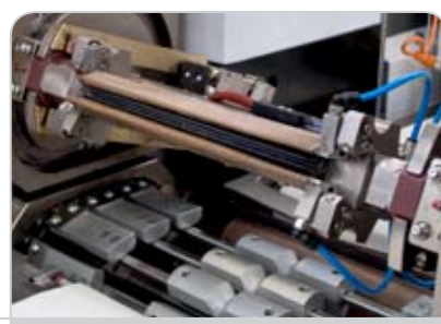
"D-Cam" type cross sealing jaw system
