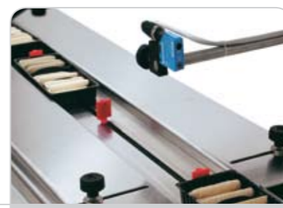
Photocell control for "No Product - No Bag" function
