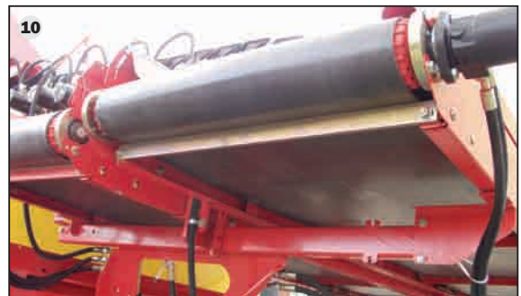
More reach: cross conveyor extension from 300 cm to 350 cm
