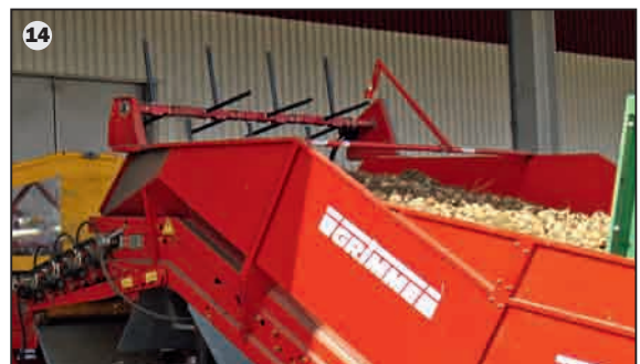
Onion distributor to loose the crop flow and ensure a gentle transfer onto the following pre-grading unit
