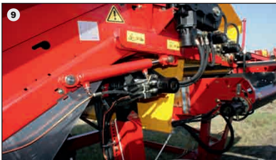
More flexible: hydraulic gap and levelling adjustment for flexible and simple adaptation to suit individual storing conditions
