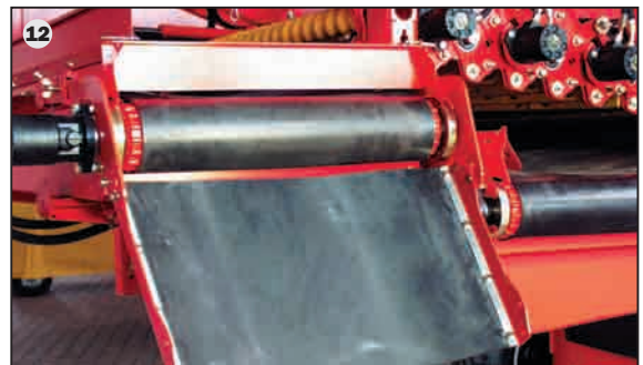
Reduced drop: Flow brake reduces the drop speed for gentle delivery into boxes.
