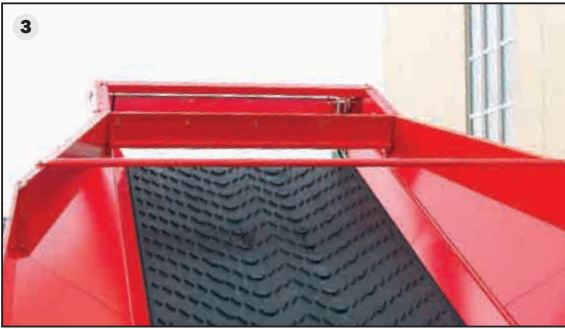
Even flow: The hopper retaining wall ensures even crop flow and a consistent feed to the following machines.
