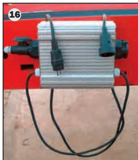
Complete control: FLOW-CONTROL (15) enables the operator to start/stop all machines in the handling line via the operator terminal. It is possible to connect all machines to FLOW-CONTROL. – If required it is also possible to connect machines from other manufacturers into the FLOW-CONTROL. If so then an AFG-box (16) is necessary.
