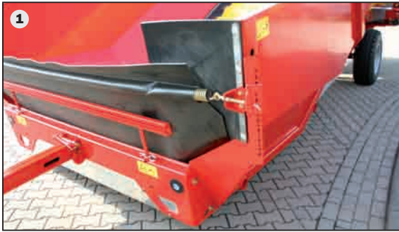
Simple: simple height adjustment to suit different trailers in steps with the spring loaded intake flap
