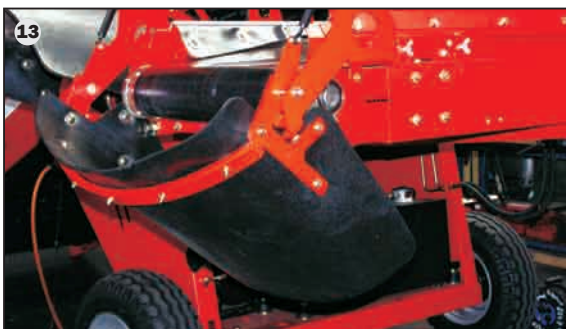
Less drop: gas cylinder operated chute to reduce the drops dramatically and even more gentle box filling
