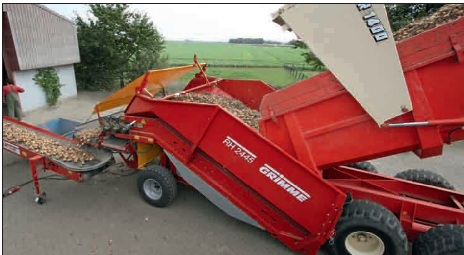
Fast emptying for increased output: The 300 cm wide intake width enables an easy moving at the intake side, and even better at the XXL-version increases the intake width to 340 cm and the hopper volume to 21 m 3 .
