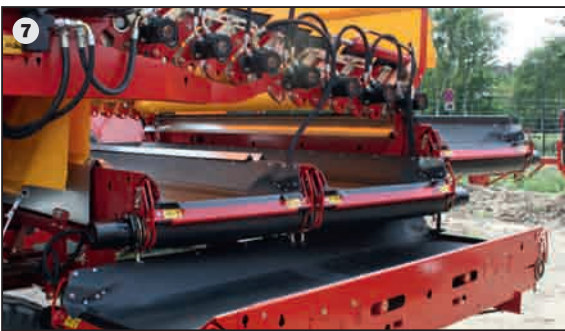
Good separation: special polyurethane pre-grading rollers for high output and gentle pre-grading. Gap adjustment is possible according to the required grading size.
