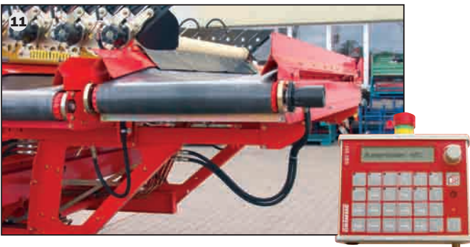
Simple solution: electrically operated "left/off/right" flow direction of the cross conveyor – optimum control via operator terminal
