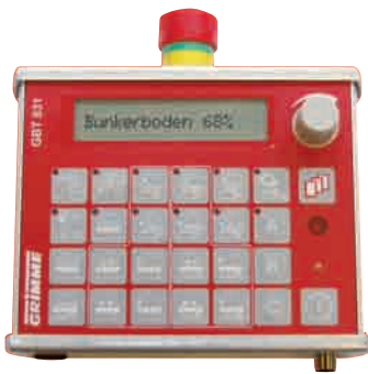
Your control centre: simple setting of the main functions via GBT – e.g. the hopper floor speed, gap and levelling adjustment of the pre-grading rollers, conveyor speed or the TURBO-CLEAN option
