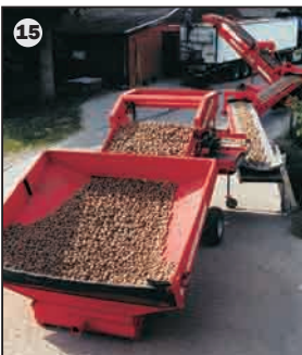
Simple solution: electrically operated "left/off/right" flow direction of the cross conveyor – optimum control via operator terminal
