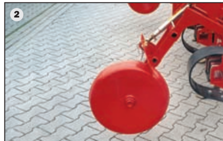
Round bodied stainless steel shaping board (option)
