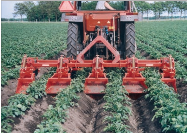
Loose soil: the individual row shaper at work
