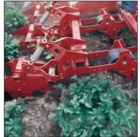
Loose soil: the individual row shaper at work
