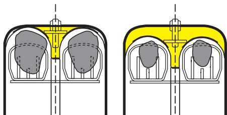
If it doesn't fit, we make it fit: the adjustable drop trunks. Narrow for small seeds and wide for large seeds.
