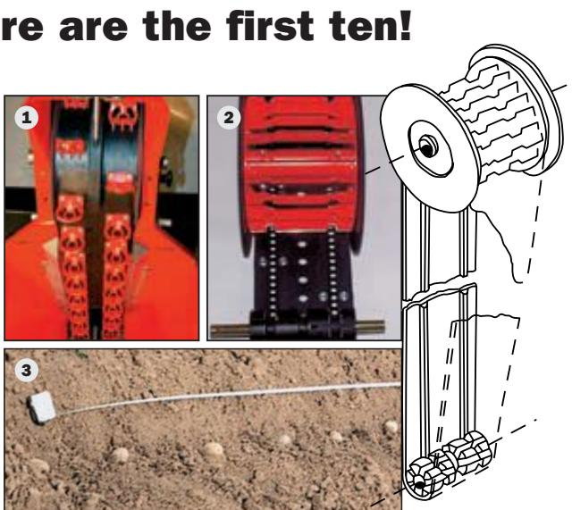
Small details which make a big difference: The large diameter upper pulley (1) ensures a positive drive and safe delivery, even with long potatoes. It also gives correct belt guiding. Two reinforced guiding ribs (2) behind the belts ensure a reliable alignment, even with oversized potatoes at the upper pulley. And the smaller belt pulley (4) at the bottom guarantees a fast opening and therefore a good delivery (3).
