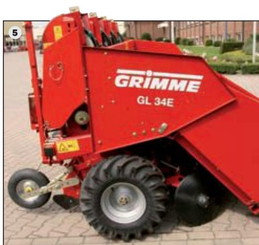
*For good running: The GL 34 E is fitted with four powerful planting elements equipped with 4 wheels (4) as standard – for optimum running also on loose soils. The compact construction ensures accurate steering of the machine.*
