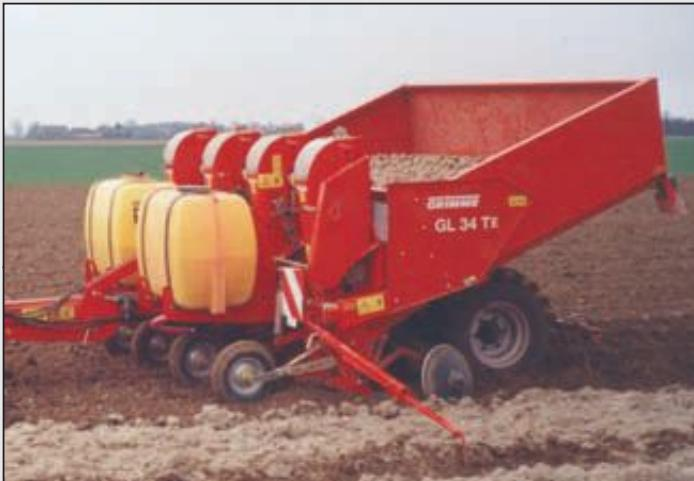
Large bunker capacity combined with small tractors: the trailed potato planter GL 34 TE with simple connection to the tractor. Easy assembling of tanks for spraying device possible (option). Furrow opener on parallelogram is standard on the machine.
