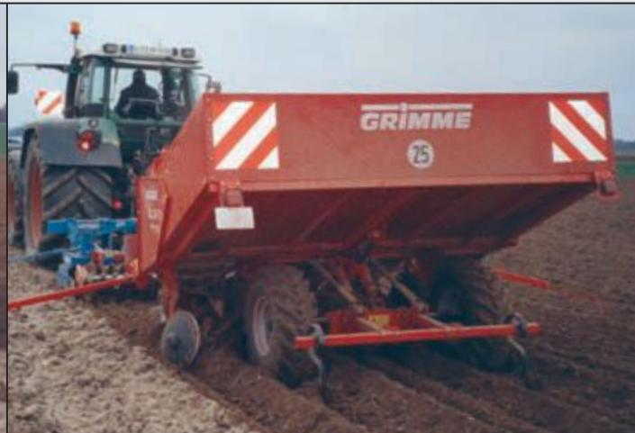
Keeping on the success line: Two bigger wheels carry the GL 34 TE behind the tractor track. Two wheels arranged between the planting elements ensure the drive. Easy filling of the tipping bunker from a trailer is possible. Another plus: the low filling height of 0.8 to 1 m.
