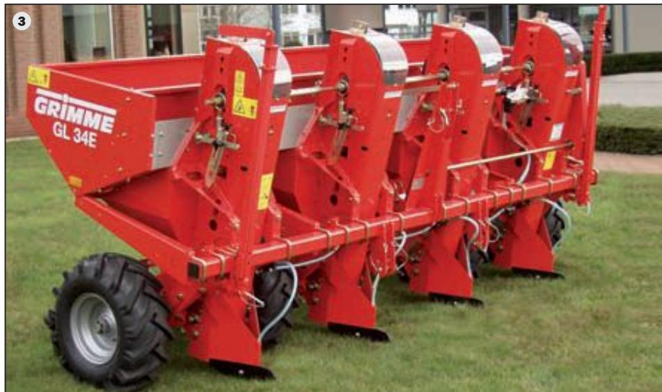
*Quickly ready: The 2- and 4-row GL 30-ECO-models are easily attached to the tractor hydraulics. Easy setting of the planting distance. With the short and compact construction it's also possible to operate the machine with a small tractor (starting at 37 kW) (3).*
