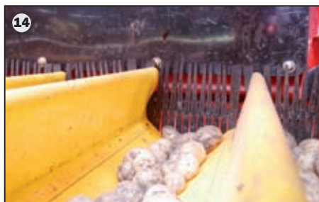
14 Patent solution for high output: The new powerful elevator construction has a 30% larger pocket volume than conventional elevator webs of the same width. Together with the patent pending active side finger combs, this ensures a smooth crop flow from the separator to the picking area.
