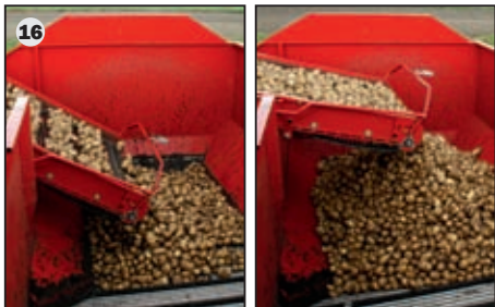
16 Professional bunker filling: The bunker filling starts directly from the bunker floor. The automatic bunker filling (option) ensures constant minimum drop heights. At the same time the bunker floor is moved forward until totally filled.
