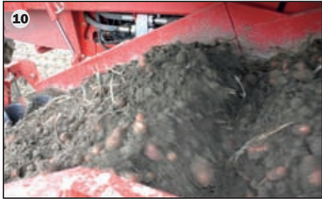
10 Controlled sieving: The extra intake web (option) increases the sieving capacity of the webs. Hydraulic speed control allows the webs to be set to their optimum for the harvest conditions.
