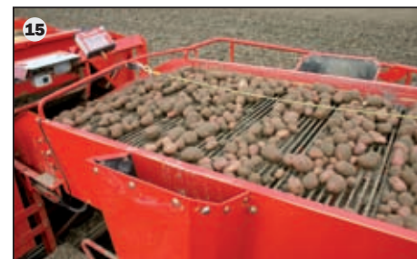
15 Well picked: The generous picking table offers the picking-crew a comfortable working place. It is possible to control main machine functions from the terminal at the picking table.
