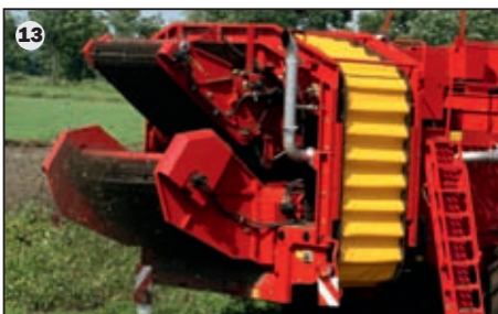
13 Good combination: In addition to the fine haulm elevator, a hedgehog web (option) named N-separator can be added on the top to separate further haulm and trash.
