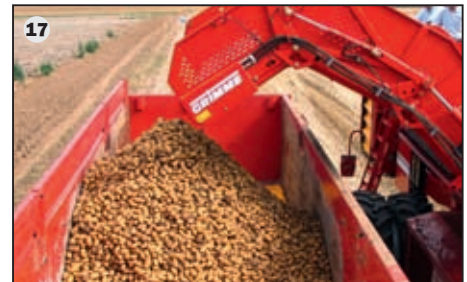
17 Gentle handling in all areas: The bunker end is hydraulically adjustable in 3 sections and reduces the drop into the trailer. Thus ensuring a minimum drop into trailers, independent of the trailer height, and also allows unloading whilst harvesting.
