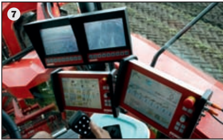
7 Under control: simple operation of the harvester with the standard touch screen VISUAL-CONTROL VC 100. The chassis and engine operations are controlled from the GBT 2100. Alternatively a second VISUAL-CONTROL VC 100 can be specified (option) to operate the chassis and engine.
