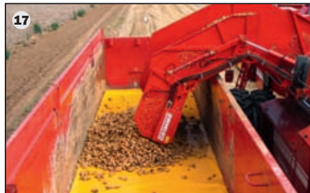
17 Gentle handling in all areas: The bunker end is hydraulically adjustable in 3 sections and reduces the drop into the trailer. Thus ensuring a minimum drop into trailers, independent of the trailer height, and also allows unloading whilst harvesting.
