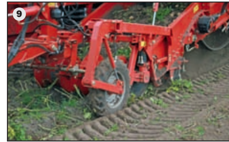
9 Extra wheel – less work: with TERRA-CONTROL (option) an additional support wheel (front left-hand side) controls the digging depth.
