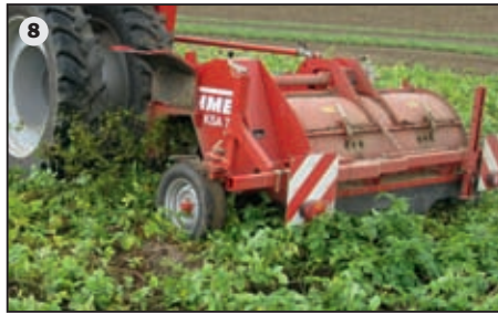
8 Pays itself: for strong conditions the robust haulm topper KSA 75-2 with cross conveyor to discharge the haulm to the side
