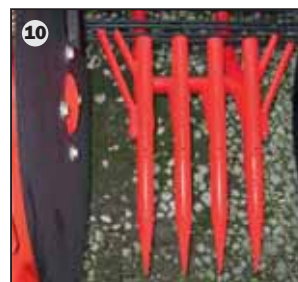
Carrot intake: large, distance adjustable support wheels, manual depth adjustment and a 1- or 2-row carrot share. Various row width and distances possible
