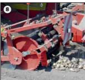
Windrow intake for light soil with centre share and rubber roller or for heavy soils with rotor shaft
