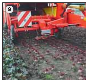
Vegetable intake: through typed share with support rollers. Special solutions are possible.
