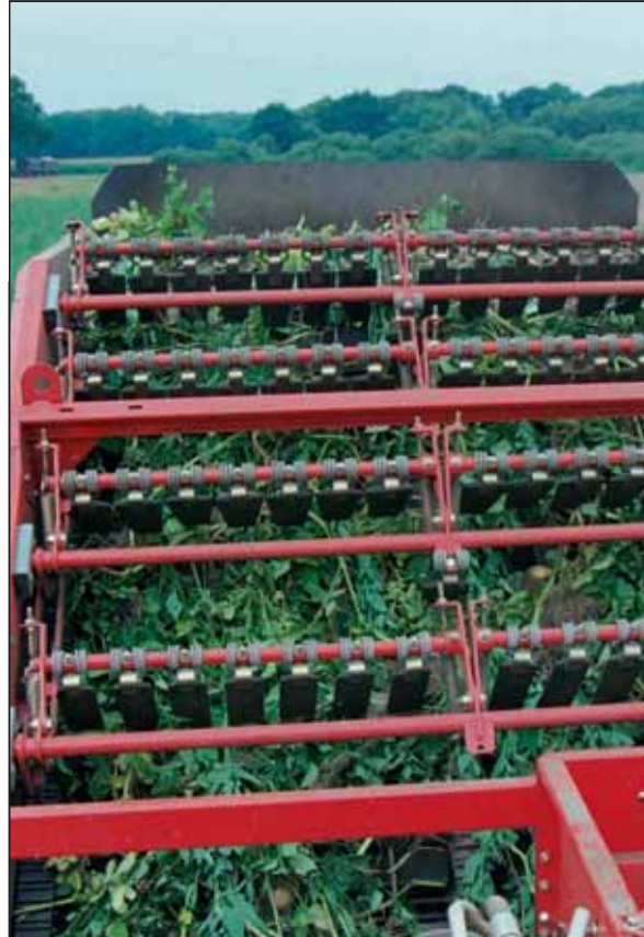
Optimum gentle crop handling: deviner web with soft polyurethane flights (distance 200 or 280 mm)
