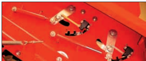
Infinitely adjustable with digital technology: the 6 back holding combs (3 on top and 3 at the bottom) on the haulm web (option)
