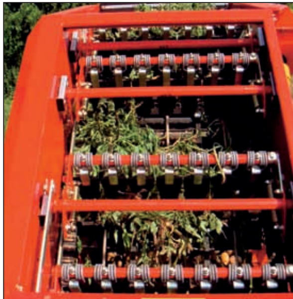
Optimum gentle crop handling: deviner web with soft polyurethane flights (distance 200 or 280 mm)
