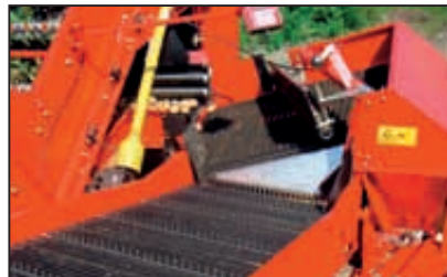
Type NB: hedgehog web and scraper roller driven from the tractor hydraulics
