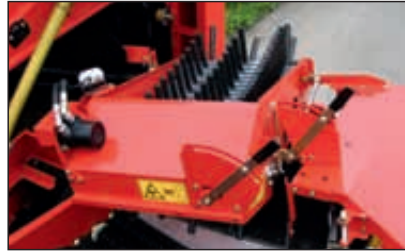
Infinitely hydraulically speed adjustment of the finger web speed
