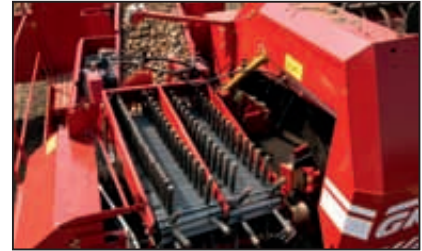
UB 900, double finger web (option): increased separation on cloddy soils
