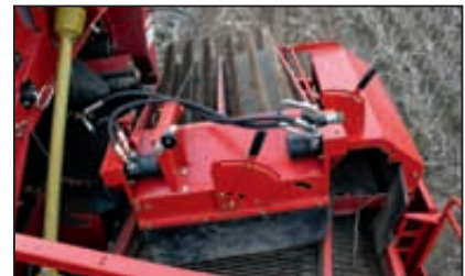
SB 900, double brush (option): increased separation on stony soils
