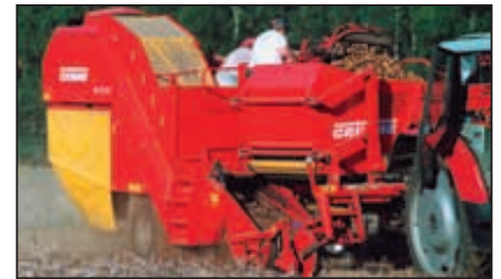
SE 75-30: for medium to large fields, compact good visible construction, moving floor bunker for 3,000 or 3,300 kg
