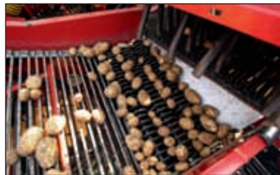
Worthwhile option: 3-grader roller
