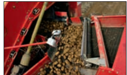
Type NB: for soils with little clods and trash
