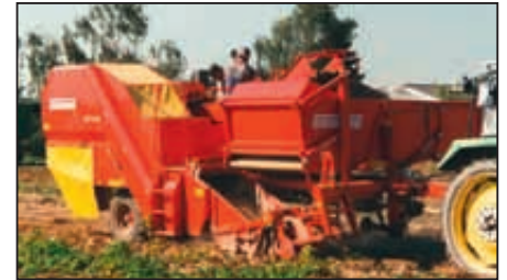
SE 75-20: for small to medium sized fields, special compact (low) construction, moving floor bunker for 2,000 or 2,300 kg
