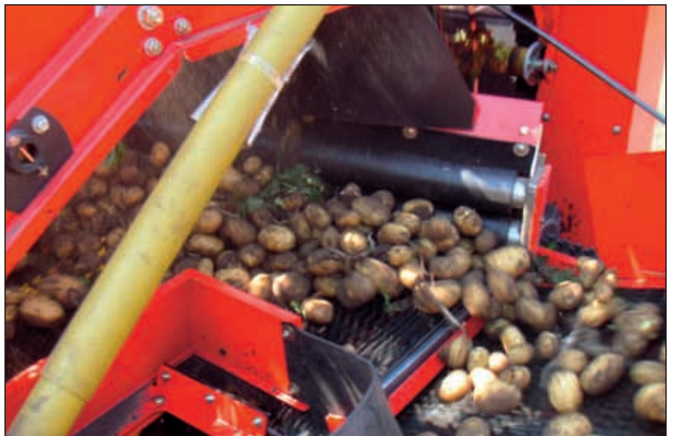
Infinitely adjustable with digital technology: the 6 back holding combs (3 on top and 3 at the bottom) on the haulm web (option)
